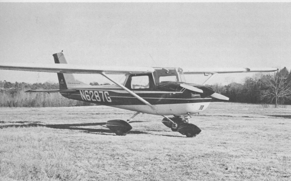
The Cessna 150 is a two-passenger aircraft specifically designed for training purposes. It cruises at about 110 miles per hour. Students pursuing their private license spend at least 40 hours in this aircraft in the college's program.
